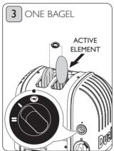
Rotate the 'selector switch' anti-clockwise to the bagel indicator.
