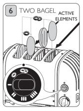
Rotate the 'selector switch' anti-clockwise to the two bagel symbol. Only the second and forth element from the left will heat up.
