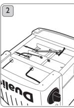
Loosen locking nuts on Unscr retaining plate using a 6.5mm wires. spanner and slide back.
