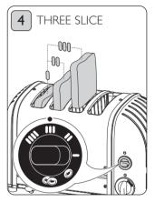
Rotate the 'selector switch' clockwise to the three slice indicator. The first three slots from the left will toast on both sides.
