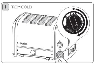
When the toaster is cold and being used for the first time set the 'timer' to the 'circle' indicator, the extra time is because the metal body will absorb some heat. After the toaster has warmed up, slightly reduce the toasting time to give consistent results.
