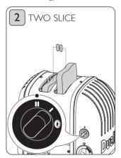
Rotate the 'selector switch' clockwise to the two slice indicator.
