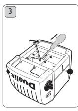
Unscrew brass links and wires.
