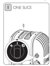
Rotate the 'selector switch' clockwise to the one slice indicator.
