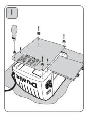
Unplug and place toaster on a soft cloth. Remove crumb tray and unscrew feet to remove the base plate.
