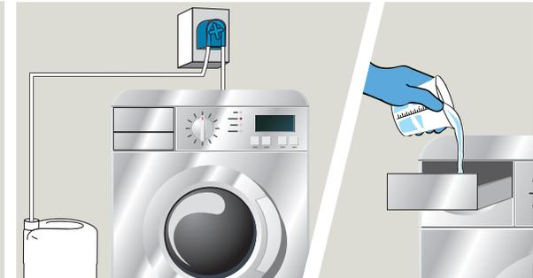
**2** Connect to an automatic dosing system. Alternatively pour into main wash dispenser.
